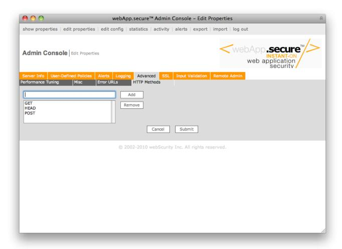
Type the name in the input box, click the "Add" button, followed by the "Submit" button to add a method to the list. Highlight a name in the list, click the "Remove" button, followed by the "Submit" button to remove a method from the list.
