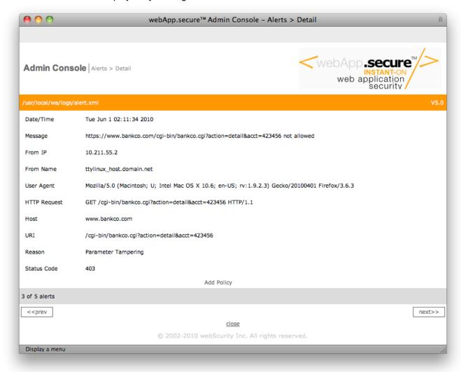
Details of a single alert are displayed when the date/time is clicked.
